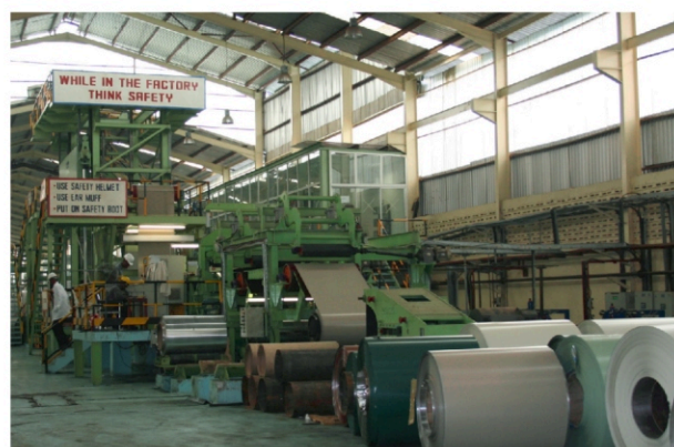
This fully automated Ultra Modern Colour Coating Line for production of ovenbaked aluminium roofing sheets, located in Ota, Ogun State, is the first of its type in Africa. Owned by Kolorkote Nigeria Limited and financed by FirstBank.
